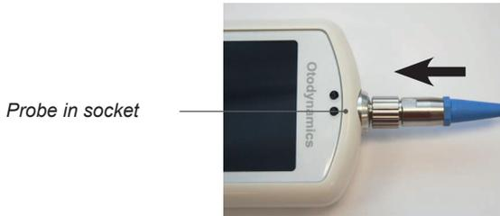
Screw up the **knurled sleeve** in a clockwise direction until finger tight.
