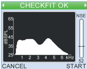
Press the left/right arrow keys during **Checkfit** to access the **Stimulus Spectrum Display**. This shows how the energy in the stimulus waveform is distributed over frequencies. This distribution is dependent on the fit of the probe and the geometry of the individual ear canal.
