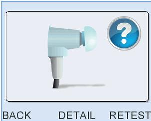
This result indicates that the probe is working and the levels recorded at all frequencies are within the absolute useable limits. The probe is still useable but there has been a change at one or more frequencies of more than +/- 3dB when compared with previously saved values for this probe. This can be due to a debris in the coupler. Replace the coupler if necessary, replace firmly into the test cavity and repeat the Probe Test.
