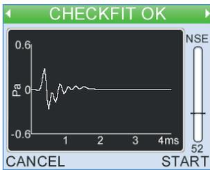
Press the left/right arrow keys during **Checkfit** to access the **Stimulus Waveform** display. This shows a real time view of the stimulus waveform. With a good probe fit the waveform should have an initial large positive then negative peak followed by a flat line response.
