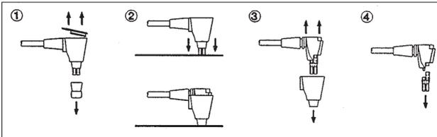
First, unplug the probe from the instrument. Remove the tip and then the lid (fig. 1). Remove the coupler tubes by pushing the end of the tubes down onto a hard surface (fig. 2). Pull out the tubes by gripping them (fig. 3). Never remove them by pulling on the cable. Finally, pull the coupler tubes away from the probe (fig. 4).
