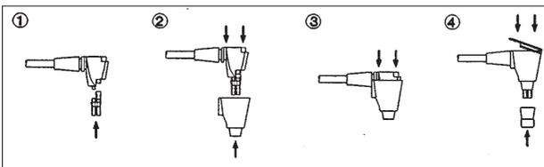
Fit the new coupler tubes to the probe assembly (fig. 1). Fit the outer shell (figs. 2 and 3), followed by the lid (fig. 4). Click the lid into place using firm finger pressure only. Finally, fit a new tip (fig. 4).
