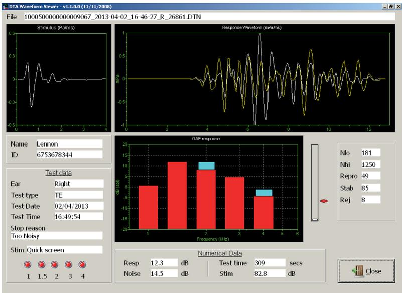
The example above is of a test was allowed to run in noisy conditions to time out. Nht is more than 3 times Nlo resulting in a stop reason of “Too Noisy”. The stimulus level is within the acceptable range but stimulus stability is only just. This means that while probe fit is acceptable, environmental noise levels were too high to detect the presence of an OAE if there was one.
