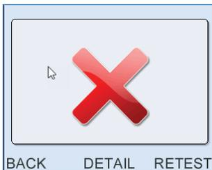
If a **Fail** is shown on screen you must inspect the probe coupler tubes again for debris which can cause this failure. Replace the coupler if you see any debris or damage. Re-insert the probe in the cavity. Repeat the Probe Test, by selecting **Retest**.
