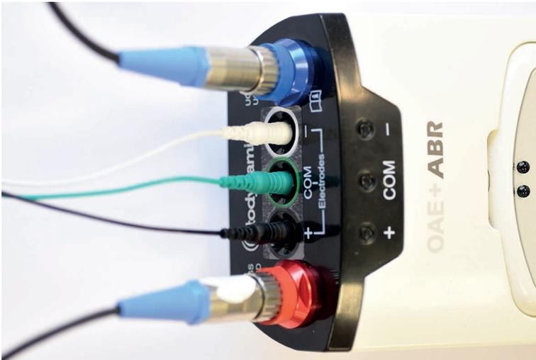
Carefully align the sensor connector plug with the appropriate sensor socket (observe colour coding) and then push in firmly.
