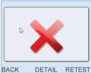
This means one or more of the stimulus levels recorded are outside the absolute limits specified for the Probe for screening use. If a **Fail** is shown on screen you must inspect the probe coupler tubes again for debris which can cause this failure. Replace the coupler if you see any debris or damage. Re-insert the probe cavity and ensure environment is quiet. The performance of probes that fail on the absolute range are not effective for screening and must be withdrawn from service.
