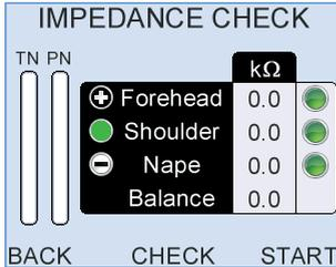
If the impedances are any higher than this, then check the connection of the cable to the test cavity and press **Check**. If after adjusting the impedances still do not show 0k Ohms then there may be a problem with the electrode cables. Remove these cables, connect alternative cables and retry.
