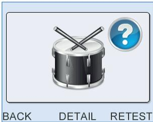
If a **Noisy** result is repeated when the room is quiet, and the probe is well fitted to the cavity, this may indicate a fault with the probe or instrument. Remove the probe from service. Use another probe. If the replacement good probe gives the same **Noisy** result, withdraw the instrument from service.
