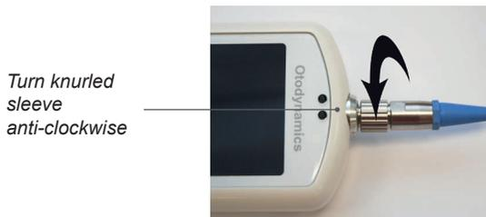
Then gently pull the probe out from the probe socket.
