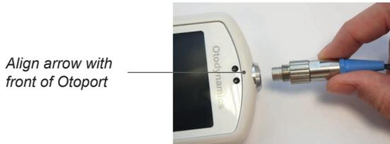
Push the probe into the socket until it hits the end stop. DO NOT force in the probe.
