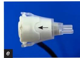
Align the semi circle key on with the TIP HOLDER with the probe body as shown here.
