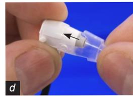
To fit the TIP HOLDER to the probe body, ensure that it is aligned with the probe head as shown above.
