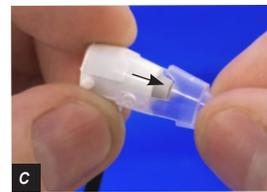
Once the TIP HOLDER tabs are unclipped. Pull the TIP HOLDER away from the probe body and discard the old TIP HOLDER.
